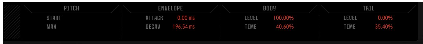
A dedicated **Envelope Values Display** is located below the curves, showing all parameter values for the currently focused envelope in one place. It allows for quick and precise centralized adjustments and easy macro control assignment (using Shift + Right-click).
