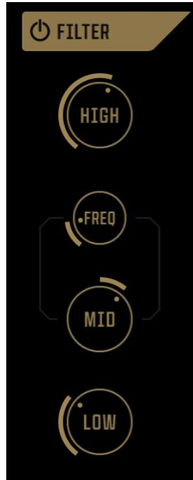
At the end of the Master chain lies a **3-band semi-Parametric Filter**, specifically engineered for Kick Drum processing. It is designed to boost low-end weight, add presence and clarity in the highs, and precisely control specific low-mid frequencies with tube-inspired coloration. The Master Filter additionally improves overall phase coherence, ensuring production-ready results that cut through the mix.
