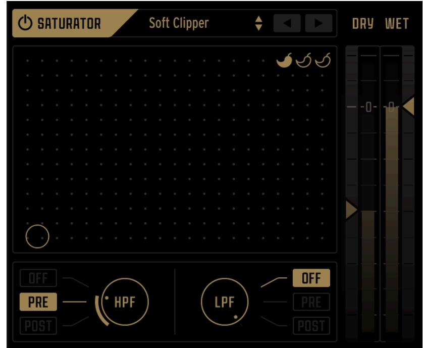
Two dedicated **Linkwitz-Riley filters** (12 dB/oct High-Pass and 12 dB/oct Low-Pass) operate on the saturated (WET) signal. Each filter can be independently enabled, tuned, and set to apply either pre- or post-saturation, enabling accurate tuning and mix control.
