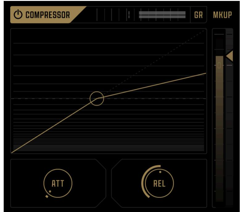
Right next to the **COMPRESSOR** button, at the top of the module, lies a Gain Reduction (GR) meter. The GR Meter displays gain reduction from 0dB to 18dB Gain Reduction, with background indicators placed at 1.5dB intervals.
