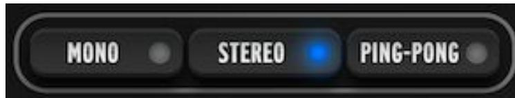
**MONO:** Left and Right input are summed and processed as one channel that feeds both the Left and Right delay units
